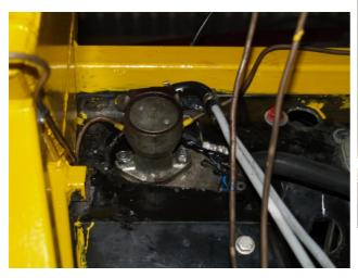
The brake master cylinder and vacuum feed are fitted; the two light pipes are the reservoir feed which needs a bracket fitting on the back of the frame. I'm going to need another coat when it's all finished!
