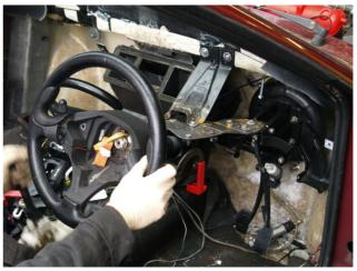
The shaft is too long; in a masterpiece of fabrication we cut and shut (TIG welding leaves a lovely finish) the thing an inch and a half short. Ooops... still, Joe has lots on his shelf!
