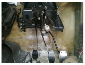
Turns out there's one place, and one place only, where it will go. There's a slight tilt to it, and I haven't worked out the clutch master yet, but it looks as if everything will fit. Three bolts and a big hole later and it's in. The throttle pedal is mounted on a couple of stand-offs (which incidentally lets me adjust the position slightly) and works its way around the steering column.
