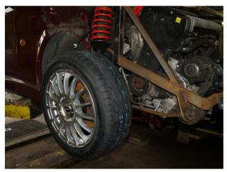
Team Dynamics; standard 108mm PCD but an offset of only 25mm which moves the wheels outwards 30mm and makes all the difference. With the slightly narrower 15/185R55 Toyo T1-R rubber it's within a couple of mm of the metalwork on full lock. Result.
