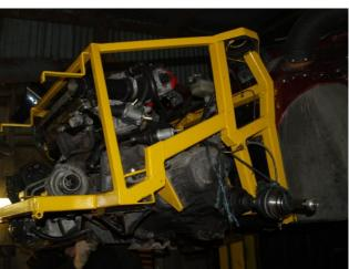
The suspension goes back on, along with a strim of steel to support a slimline fan behind the radiator. One of the many many wiring looms that Fiat find it necessary to use is fitted, and wrapped around the engine.
