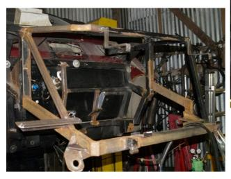
On the left is the mount for the oil cooler, and the bracing for the tiebar. While the bits are out, time for lots of yellow paint. Most of it ends up on the framework, though a bit finds its way onto the tub and a local gravitational anomoly causes a Jackson Pollock effect on Joe's floor.
