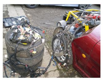
So, out with the hole cutter and some new holes appear. The looms are plugged into the fuse box, only to discover that it's the wrong fuse box... there are two or three types. Actually, it's the wrong loom, but same difference. All change, get the correct loom out of another donor. There's another loom which also plugs into the fusebox and runs front to back, and carries the lights and fuel pump feed; a fourth
